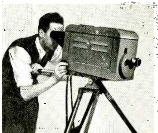
Camera built by K. A. J. Russell of Bournemouth. It uses an RCA 5527 iconoscope pick-up tube working on 250 lines (non-interlaced) and contains a pre-amplifier, a line amplifier and a viewfinder.
