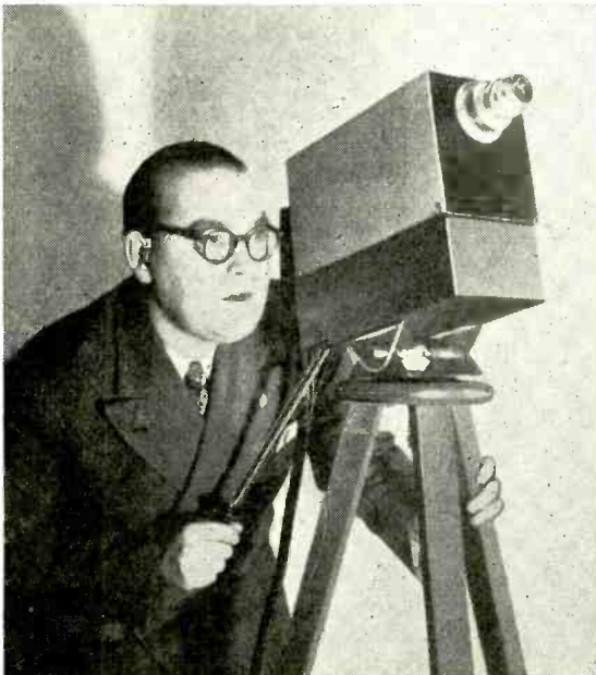
Camera built by B. Cederqvist of Helsinki. It contains an RCA 5527 pick-up tube and an amplifier using miniature valves. The deflection circuits for the pick-up tube are housed in a separate unit.
