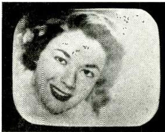
Television picture obtained with Mr. Russell's camera (see above). The subject, an advertisement photo, was illuminated by two 500-watt photoflood bulbs and this picture was taken from the screen of a 9-in monitor tube.
