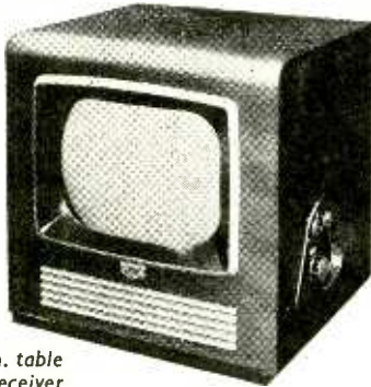
Cossor a.c./d.c. television set model 927 with 12-in. tube.
