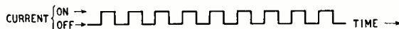
Fig. 3. The maximum current frequency of binary signals (i.e., current on or off) occurs when all the odd signals are of one kind and all the even signals of the other. An unending sequence of this kind has zero bandwidth and conveys no information.
